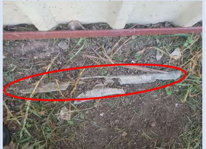
Photograph 10 Asbestos fragments in soil
